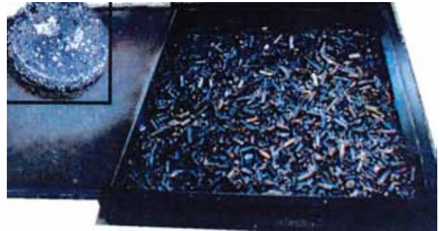
60 minutes later, 97% recyclable brass and lead ready for recovery
